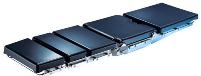
OR table-top for head surgery 1150.25: Maximum of five sections with head plate, two-part back plate, seat plate and fixed leg plate. Motor-powered longitudinal shift of 275 mm, plus motorised back plate up/down. Leg plate may be tilted downwards manually using pressure-assisted brakes. OR table-top with integral foam padding
