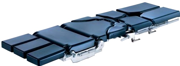
Universal table-top for traumatology and orthopedics 1150.20: Maximum of ten sections. Back plate may be tilted through ca. 70° using motor. Seat plate with two separate removable corner pieces. Removable leg plate pair, and two extension bars each with two revolving joints, and basic accessories. PUR padding; also available with SFC padding.
