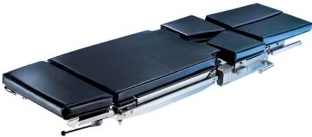
OR table-top for general surgery and MIS 1150.22: Six sections with head plate, trunk plate and four-part leg plate/knee crutch combination Maquetmatic. Table-top with power-driven longitudinal shift of 475 mm. Maquetmatic is integrated into the table-top with four individually removable sections. One-hand operation for the control of combined up/down movements.
