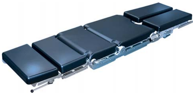
Modular universal surgical table-top 1150.30: Universal operating table-top for a wide range of applications. Comprises a seat section and a lower back plate for modular assembly to suit a number of surgical disciplines. Made of nickel-chrome steel with guide tracks and guide rails for X-ray cassettes. Automatic zero position for all motorised functions.
