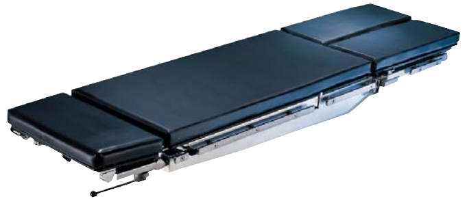
OR table-top for urology, orthopedics and vascular surgery 1150.23: Two-section trunk plate with manual pressure-assisted adjustment of back plate by ca. 30°. Table-top with power-driven longitudinal shift of 400 mm. SFC padding.
